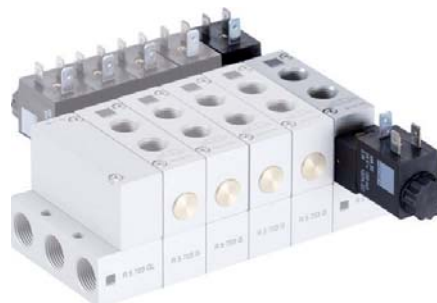
5/3-way solenoid valve with spring return to middle position, actuated by permanent signal. Ports 2 and 4 are in the valve, ports 1, 3 and 5 in the manifold plate.
